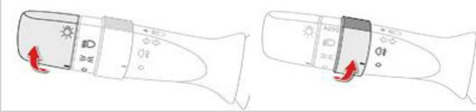
**Headlights:** rotate the dial at the end of the lever left of the steering wheel forward two clicks to operate the headlights (regular lights for nighttime driving). Pull the lever towards you to briefly engage the high beams. Push the lever towards the dashboard for continuous high beams. Pull the lever a second time to turn off the high beams.
