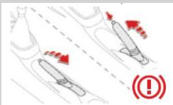
To release the handbrake pull the lever up slightly and push the button at the end. You can then lower the handbrake lever. If the
