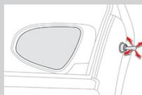
To be adjusted manually (use the controls to set the mirrors to the desired position).
