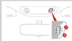
To unfold or fold the roof, press the unfolding (1) or folding switch (2) on the car ceiling, above the mirror.
