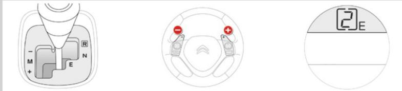
**Automatic transmission** (easy): pull the gear lever back (with the brakes applied) to select this setting (**E**).
