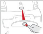
Press the black button on the hatch, and open the boot with the handle.
