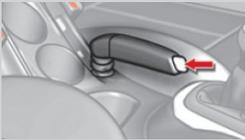
To release the handbrake pull the lever up slightly and push the button at the end. You can then lower the handbrake lever. If the handbrake is engaged whilst riding, a red warning sign lights up on the dashboard. Release the handbrake immediately!
