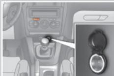
There is a socket near the central compartment, below the air conditioning controls. There is a second socket at the armrest of the rear seat, and one in the boot, on the left.
