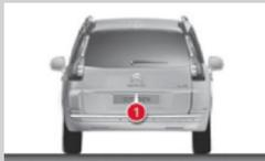
Normal operation. To open, pull the handle (1) at the base of the hatch.
