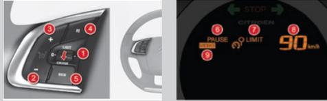
The controls are located on the steering wheel's left side:
