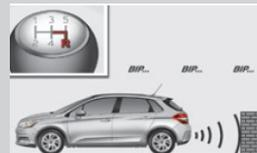
This vehicle features a park assist system in the rear. A buzzer will beep faster as you get closer to an obstacle.
