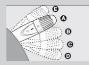
Rotate the dial forward one click to operate the rear wiper. To activate the rear washer push the lever towards the dashboard (non continuous mode).
