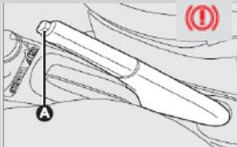
To release the handbrake pull the lever up slightly and push the button at the end. You can then lower the handbrake lever. If the handbrake is engaged whilst riding, a red warning sign lights up on the dashboard. Release the handbrake immediately!
