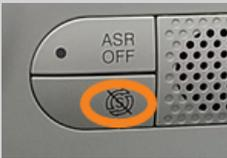
The start/stop function engages when you start the engine and you drive at least 10 km/h.
