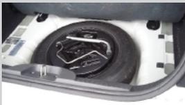
The spare wheel is stored under the boot floor, along with a jack and wheel wrench.
