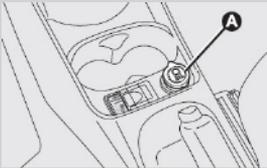
There is a 12 Volt socket in the central console, below the gear lever on the left.
