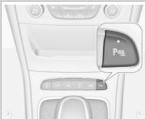
Push the park assist button to activate. The LED in the button lights up when active. Sensors measure the distance between the vehicle and any obstacles behind you. A beep will sound if you come too close.
