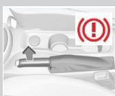
To release the handbrake pull the lever up slightly and push the button at the end. You can then lower the handbrake lever. If the handbrake is engaged whilst riding, a red warning sign lights up on the dashboard. Release the handbrake immediately!
