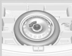
A spare wheel is stored under the boot floor, along with a wheel wrench and a jack. See instruction manual for further instructions.
