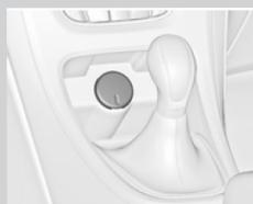
There is a 12 Volt socket in the central console, in front of the gear lever.
