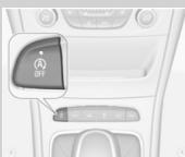
This car has a start/stop function to reduce fuel consumption. When you stop for a red light or in traffic, and you put the gear lever in neutral and release the clutch pedal, the engine will turn off automatically. The engine turns back as soon as you engage the clutch pedal. Use the button (A off) to deactivate this function.
