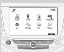
Press the NAVI button on the bottom left. Then use the multifunction button as shown on the image to select and confirm. Select by rotating the central dial, confirm by pushing the same button.
