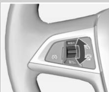
The speed limit panel is located on the left side of the steering wheel.
