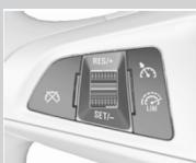
The cruise control panel is located on the steering wheel's left side.
