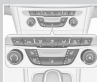
To turn on the air conditioning press the A/C button on the far left.
