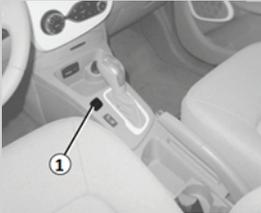
Eco Mode is a function that optimizes the range of the vehicle but impacts speed, acceleration, heating, etc. The lower part of the dashboard lights green when eco mode is active. Press the **ECO** button next to the gear selector to turn eco mode on or off.
