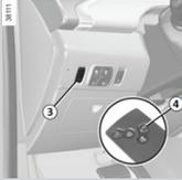
There is a charging socket at the front of the car. Connect the charging cable to the car and press the button on the key (4) or the button left of the steering wheel (3). If the cable has been attached correctly you will hear a slight hum.
