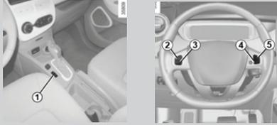
Use the switch next to the gear selector (1) to operate both the speed limiter and cruise control.
