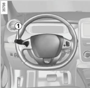
**Headlights:** With the engine running, the headlights turn on automatically during the day without having to operate stalk 1. They turn off automatically when the engine stops.
