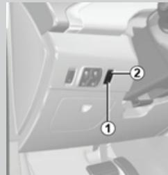
Electric cars are remarkably quiet. This system allows you to warn pedestrians and cyclists. The system is activated automatically when your speed is between 1 and 30 km/h. With the engine running, press the switch (1) to turn the function on or off. The integrated warning light (2) indicates if the function is on or off.
