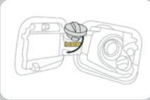
On the driver's side at the back. You can place the cap in the dedicated holder on the fuel lid while fueling.
