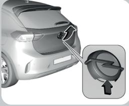
Boot switch is located under the brand symbol on the boot lid
