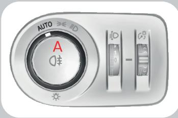
Controls on the dashboard left of the steering wheel. By turning the knob you can select between automatic, marker lights and dimmed lights.
