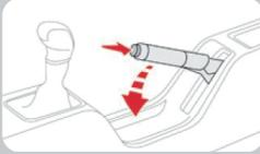
To release the handbrake pull the lever up slightly and push the button at the end. You can then lower the handbrake lever.
