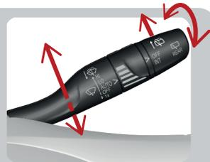
Push the lever away from you to spray and sweep. Turn the ring on the end of the lever to activate the rear wiper.
